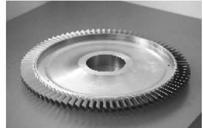
High pressure compressor disk made of Timetal-834
