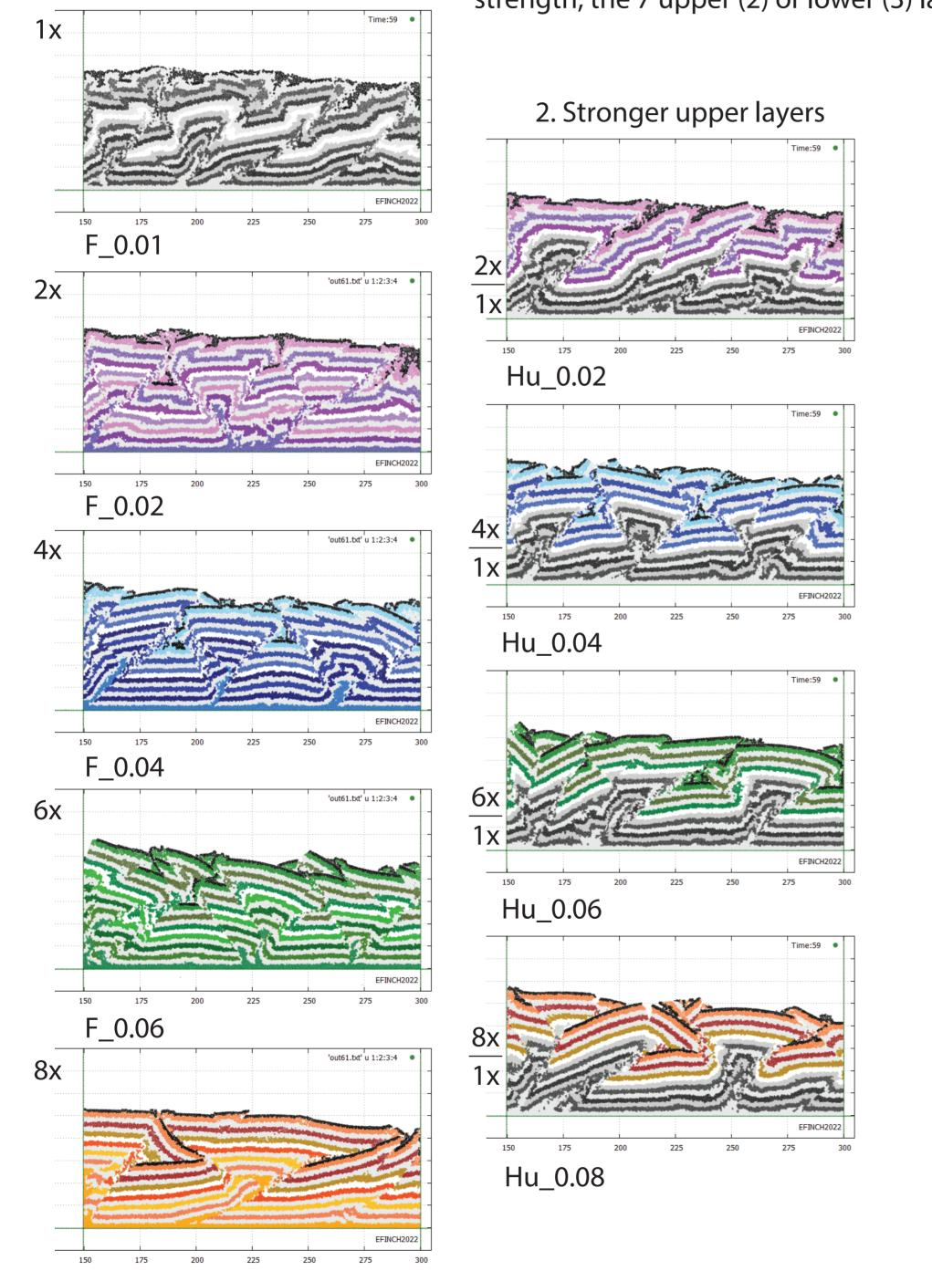
Experiments are shown where (1) the elements have the same breaking strength, the 7 upper (2) or lower (3) layers are relatively weaker or stronger.
